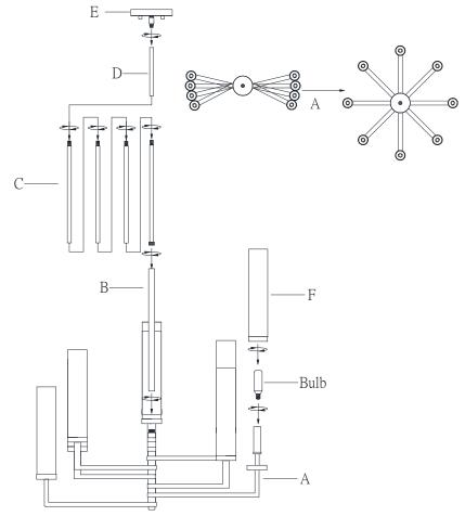
$B \to A \to C \to D \to E \to BULB \to F$
